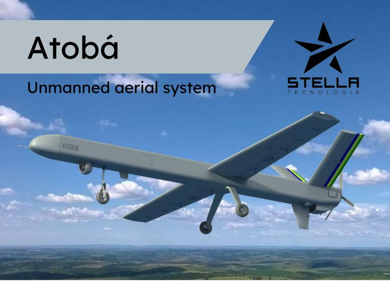
The Atobá is a next-generation Medium-Altitude Long-Endurance (MALE) Unmanned Aerial System (UAS) engineered for tactical and strategic operations. With a 500 kg maximum takeoff weight, it delivers extended endurance of 28 hours with a 75 kg payload or 20 hours carrying 150 kg, making it a mission-critical asset for intelligence, surveillance, reconnaissance (ISR), electronic warfare (EW), and beyond.
